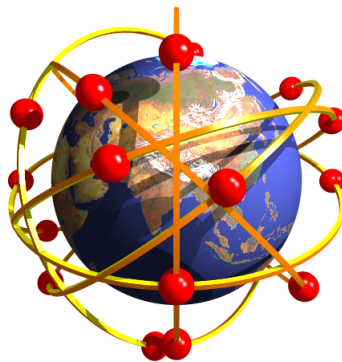
FIGURE 1. The global positioning system GPS uses the fact that a receiver can get the difference of distances to two satellites.
