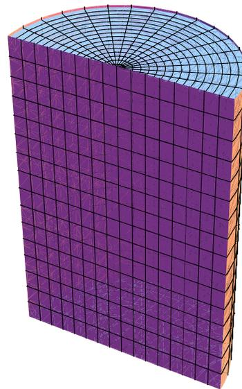
For a fixed volume  $y\pi x^2/2 = \pi/2$ , we want to minimize the material cost  $\pi xy + \pi x^2 + 2xy$ . In other words, we want to minimize the function
